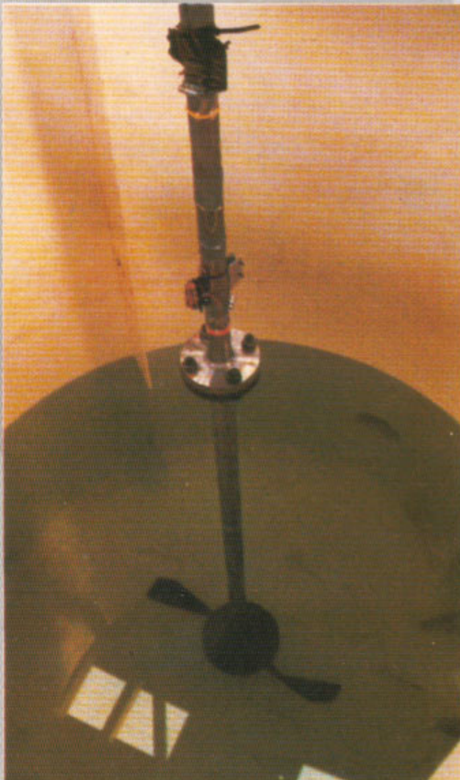
Laboratory strain gauge analysis on new impeller
